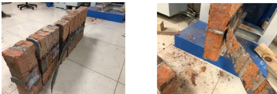
Figure 9. Failure mode of S-S1-L1 [31]
