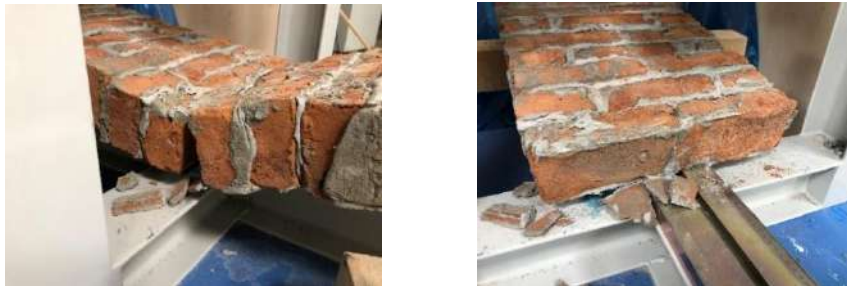
Figure 8. Failure mode of control specimen [31]
